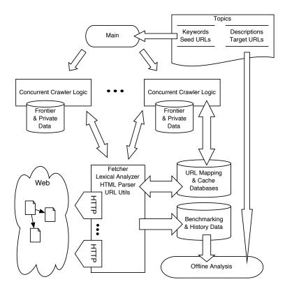
Fig. 1. Architecture of crawler evaluation framework.
