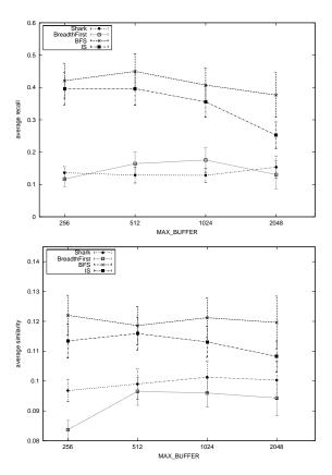
Fig. 13. Scalability of average target recall (top) and of similarity to topic descriptions (bottom) with MAX\_BUFFER by the Breadth-First, Best-First, Shark-Search and InfoSpiders crawlers.
